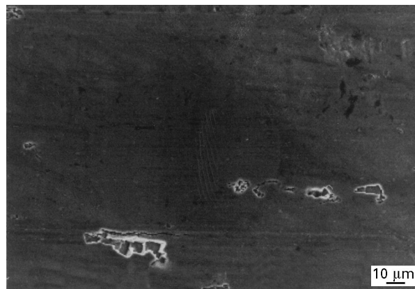
Figure 2 Micrograph of the 1199 alloy after 4 h immersion in the ASSET solution, × 500.
